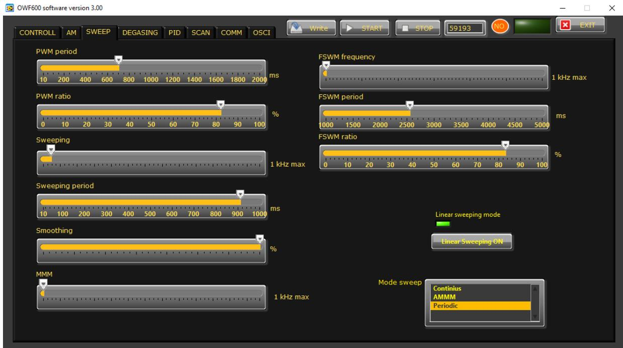
**PWM Period** – Here you can set a kind of ON/OFF working regime of the generator with the desired period in *ms*.
